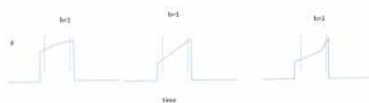
Figure 2: Airway or trans-pulmonary pressure (P) over time during volume controlled mode at constant flow inflation (not shown).
